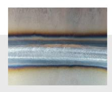
LSA (low spatter and low heat input)
